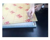
2.Use supplied suction cap to pull out the acrylic face, careful not to drop it on the ground.
