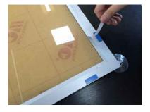
4. Remove sections of double sided tape on each corner.
